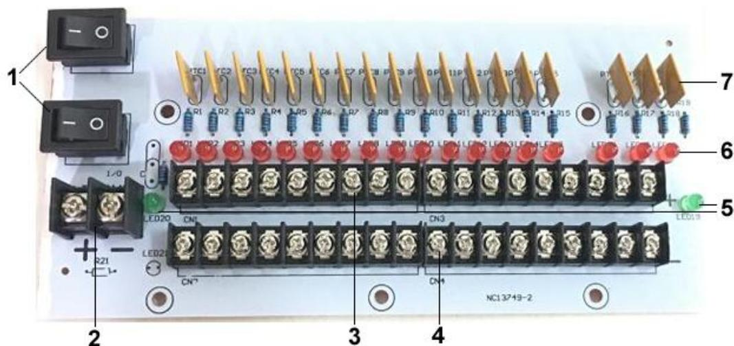
1. Power switch, used to control circuit opening and closing
