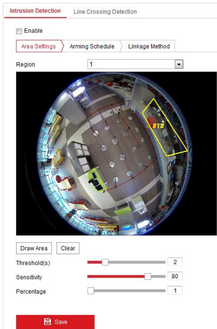
Figure 6-55 Intrusion Detection Settings
